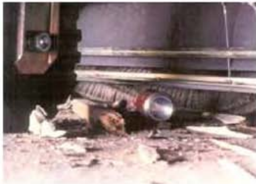
Dust flap for large debris collection
