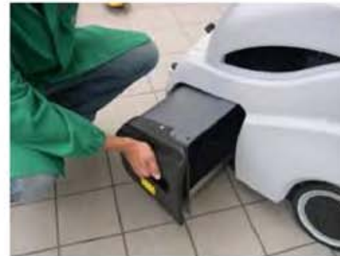
Light weight hopper material to allow easy dumping
