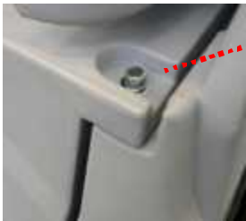
Unscrew bolt to tilt recovery tank sideways
