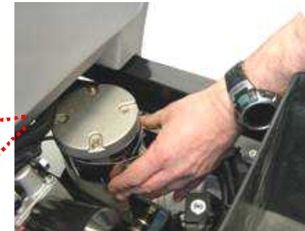
Brush motor carbon brushes replaced without tools
