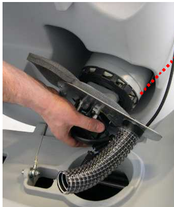
3 bolts to remove vacuum fan
