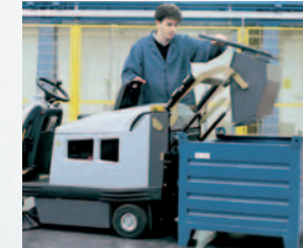
Hand-assisted high dump up to a maximum height of just over 3 ft.
