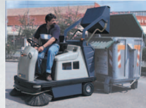
Dump at any height (up to almost 5 ft.) with large capacity waste hopper.
