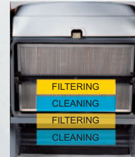
Self-cleaning dust filter is periodically cleaned by a system that automatically turns off the vacuum before shaking the filter.
