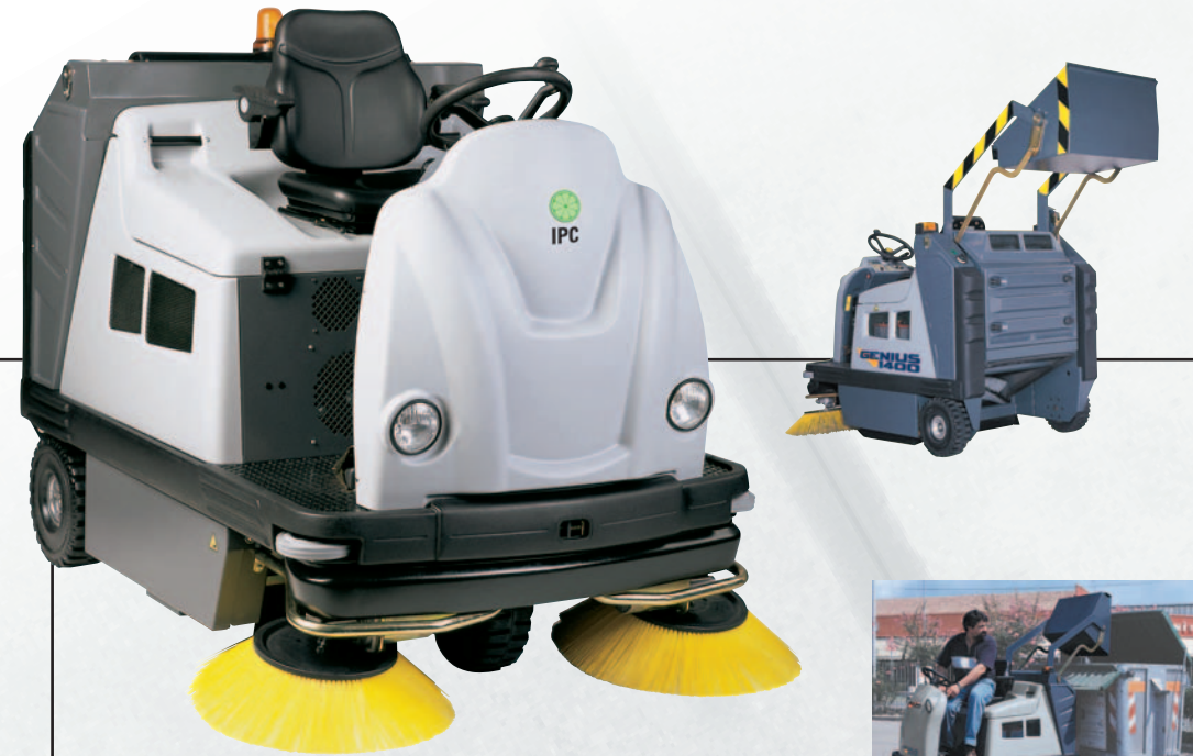
Dump at any height (up to almost 5 ft.) with large capacity waste hopper.
