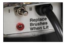
The Dual Speed model has a simple switch to change from 180 to 320 RPM. Also, there is an indicator light that illuminates when the carbon motor brushes need replacement.
