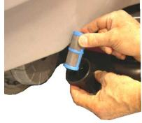
Both filters are easy to remove for cleaning
