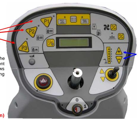
3 independent programs allow best settings for all types of applications. Solution flow remains adjustable at any time
