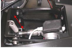
Constant brush pressure with immediate reaction. Avoids also excessive brush and actuator wear.
