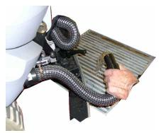
Immediate clean solution discharge if necessary with 1.5" (40 mm.) diameter hose.
