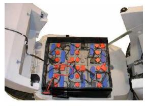
Extremely large battery compartment allows batteries of up to 325 Ah (5 running time)
