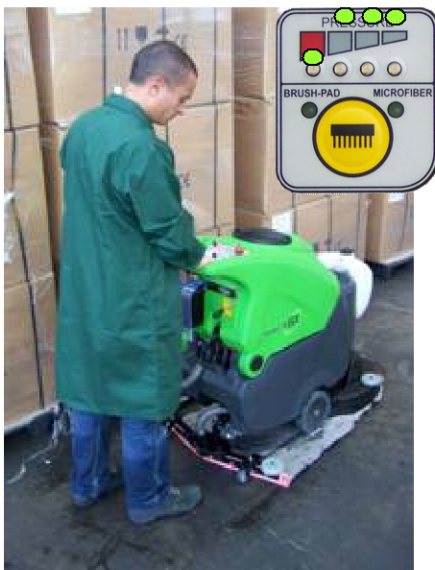
Traditional brushes or pads (200 rpm / .3-.4 gallons /min) 18-24 gallons per hour
